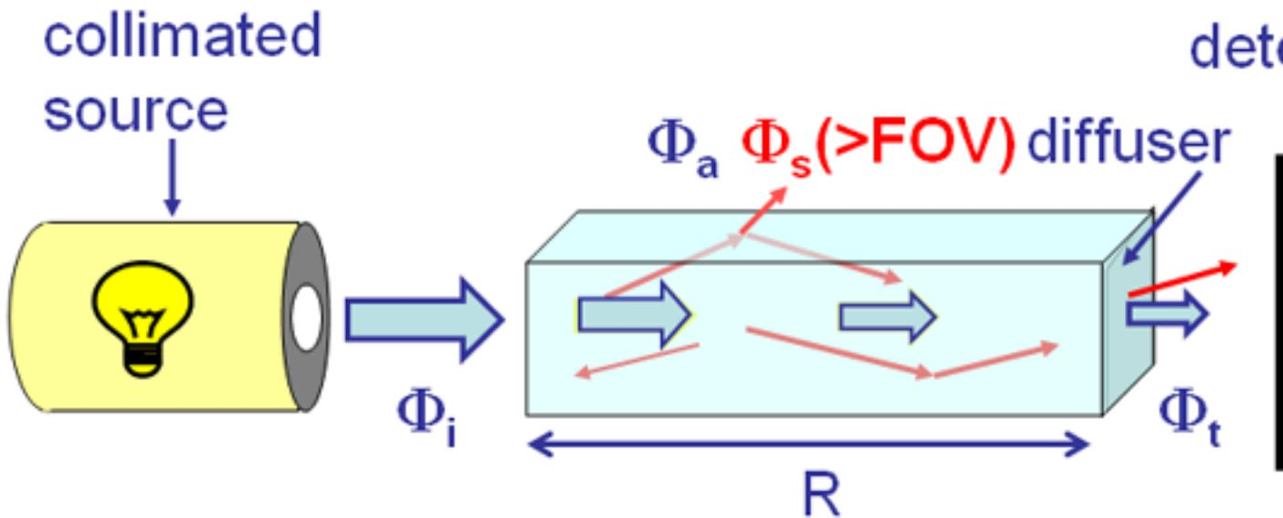
Figure 3: Schematic instrument design for measurement of the absorption coefficient  $a$ .  $\Phi_s(>FOV)$  represents the power lost to the detector by scattering into angles greater than the detector field of view.
