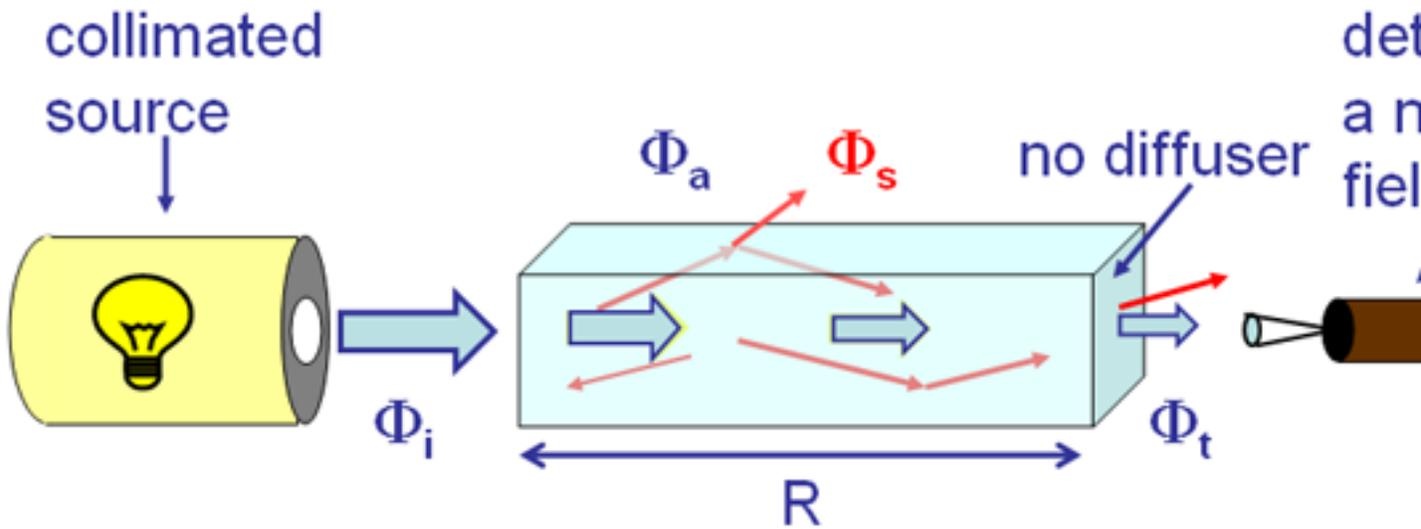
Figure 2: Schematic instrument design for measurement of the beam attenuation coefficient  $c$ .  $\Phi_s$  represents the power scattered into all directions, as indicated by the red arrows.
